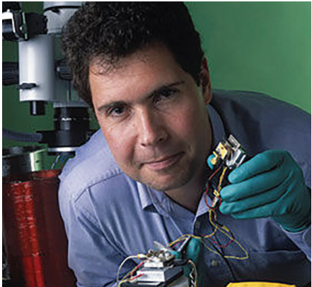
NIST physicist John Kitching displays the heart of the world's smallest atomic clock. This "physics package" is about the size of a grain of rice.
