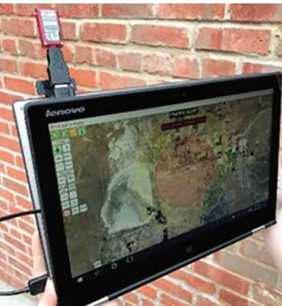
NASA AFRC’s Sense-and-Avoid System with ADS-B Avionics can be used on a portable tablet computer, such as the one shown here, with an ADS-B receiver attached. (Vigilant Aerospace photo)
