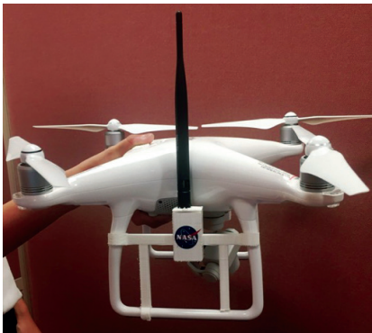
A small UAS equipped with a transponder is prepared for use in flight testing of NASA AFRC’s Sense-and-Avoid System with ADS-B Avionics with smaller aircraft. (NASA photo)
