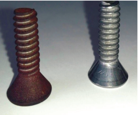
Uncoated (left) and aluminum coated (right) screws after exposure to salt spray. Corrosion is clearly visible on the uncoated screw.
