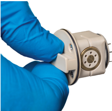
The heart of the 908 Devices product line is composed of ORNL-developed ion trap mass analyzers that are a thousand times smaller than those in conventional mass spectrometers. These diminutive traps can operate much closer to atmospheric pressures and enable the use of dramatically smaller pumps, ionizers, detectors, and electronics than in laboratory or transportable mass spectrometers. (Photo courtesy of 908 Devices)
