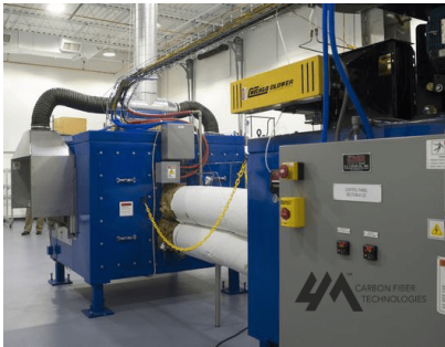
The Atmospheric-Pressure Plasma Oxidation Oven in the Knoxville-based facility owned by 4M Carbon Fiber Corp.
