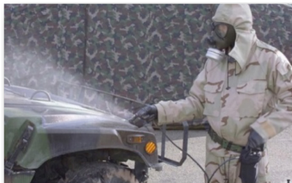
An example of a spray application of the Dahlgren Decon decontaminant.
