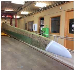
The first of the National Rotor Testbed blades is undergoing static and load testing at the NREL.
