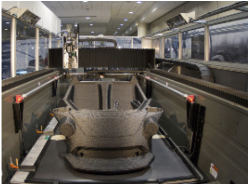
The BAAM-CI system as seen from the inside. (Photo by Cincinnati Incorporated)
