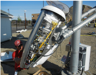
PNNL's thermochemical conversion device is installed in front of a concentrating solar power dish. The device converts natural gas into the more energy-rich fuel syngas, which power plants can burn to use less fuel and reduce greenhouse gas emissions.
