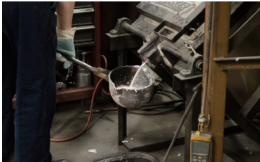
Alloyed metals are shown being poured from a furnace into a ladle to be used for filling molds.
