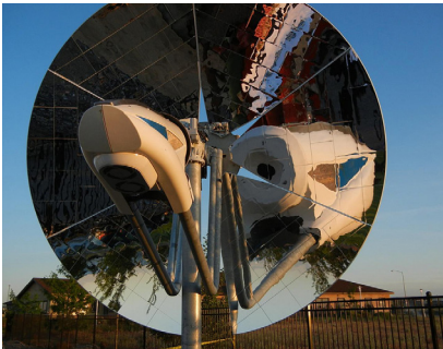
A close-up look at STARS. A single solar thermochemical plant with 200 solar concentrators on about 4 acres of land is expected to produce 1,500 kilograms of hydrogen per day, which is sufficient to supply a busy fuel-cell-vehicle filling station.
