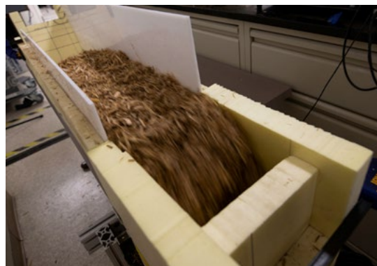
Above: A prototype conveyor at Los Alamos National Laboratory moving bulk material and measuring moisture content.
