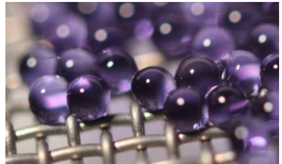
Above: Microcapsules with biodegradable shells can deliver therapeutics through a syringe. Microcapsules with gas-permeable polymer shells filled with a sodium carbonate solution, pictured above, act as mini-reactors and a storage unit to draw CO 2 from power plants or manufacturing operations much faster than approaches using unencapsulated materials and leave only non-toxic sodium bicarbonate as a byproduct.
