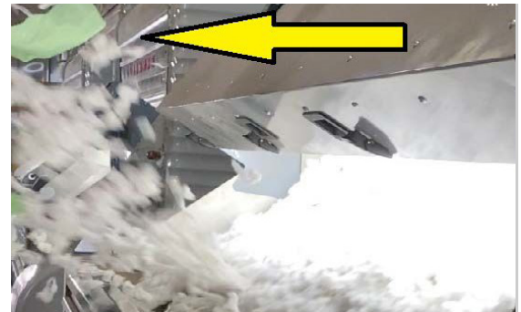
Above: The VIPR system blows the green piece of plastic detected (highlighted by the yellow arrow) out of the process stream prior to entering the gin stand.
