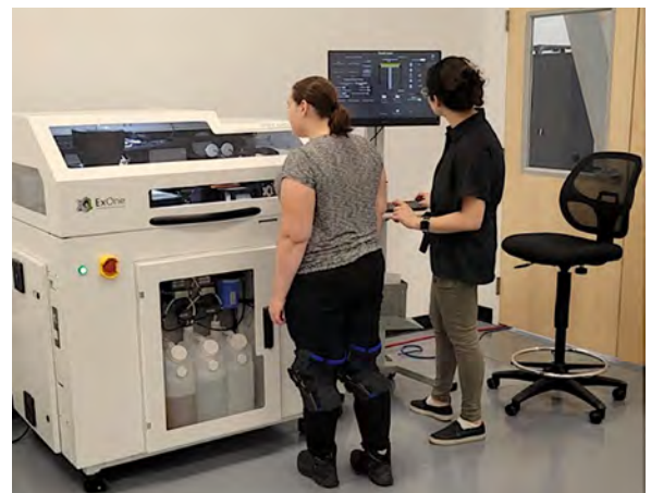
Two USNC staff members operate a small-scale silicon carbide binder jet printing system at USNC's Advanced Ceramics Manufacturing facility in Salt Lake City.
