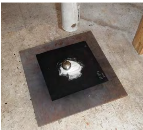
Treating triacetone triperoxide with Silent Spring prevents the violent reaction that would normally occur when a 1.8 kg steel ball is dropped 7 feet onto a 15 g sample of the explosive.
