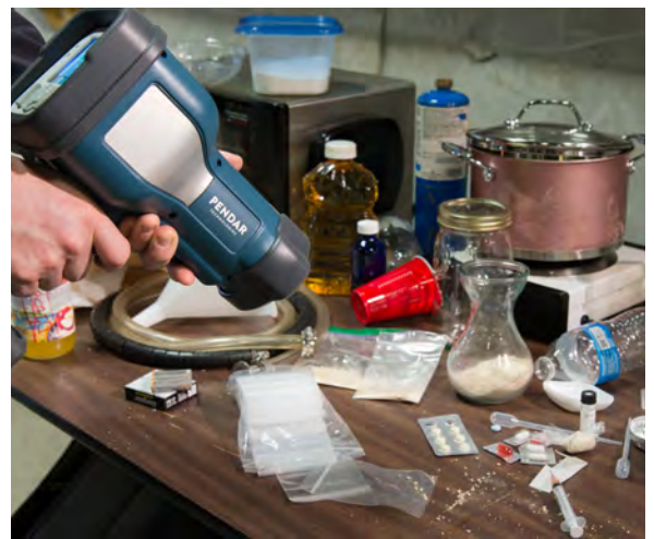
The Pendar X10 reads and identifies a variety of hazardous threats.
