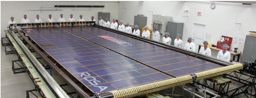
The Air Force Research Laboratory Space Vehicles Directorate— in partnership with NASA, Deployable Space Systems, Inc., LoadPath, LLC and Hall Composites—developed the roll- out solar array.
