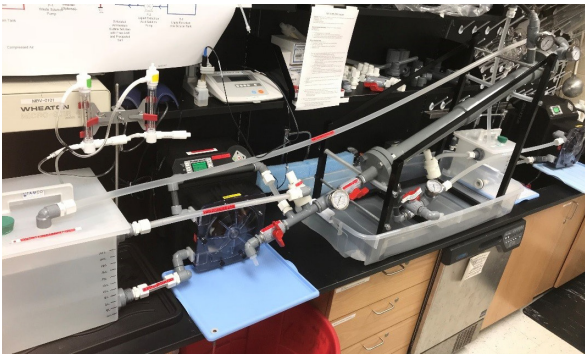
Above: Ammonia recovery from wastewater with gas-permeable membranes.
