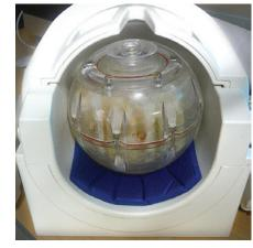
NIST-developed diffusion phantom placed in a "head coil" used for magnetic resonance imaging of the human brain.
