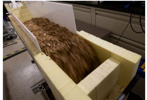
Above: A prototype conveyor at Los Alamos National Laboratory moving bulk material and measuring moisture content.
