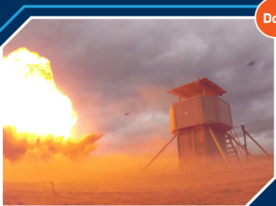
DoD | Geotechnical and Structures Laboratory Rapidly Deployed Modular Protective System Guard Tower for Counterinsurgency Operations
