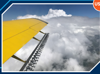
USDA | Aerial Application Technology Research Unit | Agricultural Research Service Aerial Electrostatic System for Weather Modification
