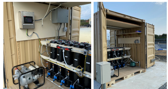
Above: The PETS System Below: The PFAS Water Treatment Research Reactor (PWTRR)
