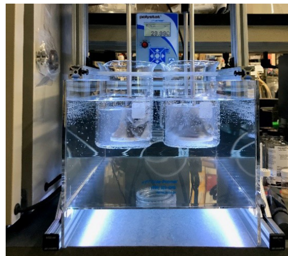
Above: A miniaturized laundry testing apparatus is used to test new surfactant molecules in real-life laundry wash conditions. Each glass beaker is filled with a small amount of water, detergent, and pre-stained fabrics. Backlighting allows for researchers to see issues during the wash cycle, such as cloudiness that is a result of incompatibility with hard water.
